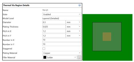
Transferred to Simcenter Flotherm XT as Cuboid representation of the Via array with orthotropic material properties to model thermal effect.
