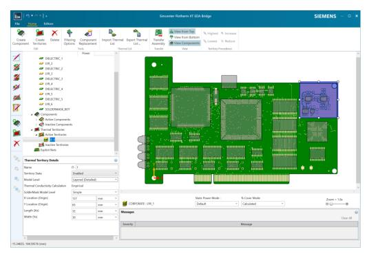
• Allows the user to define any region of a board to obtain accurate representation of local copper coverage.
