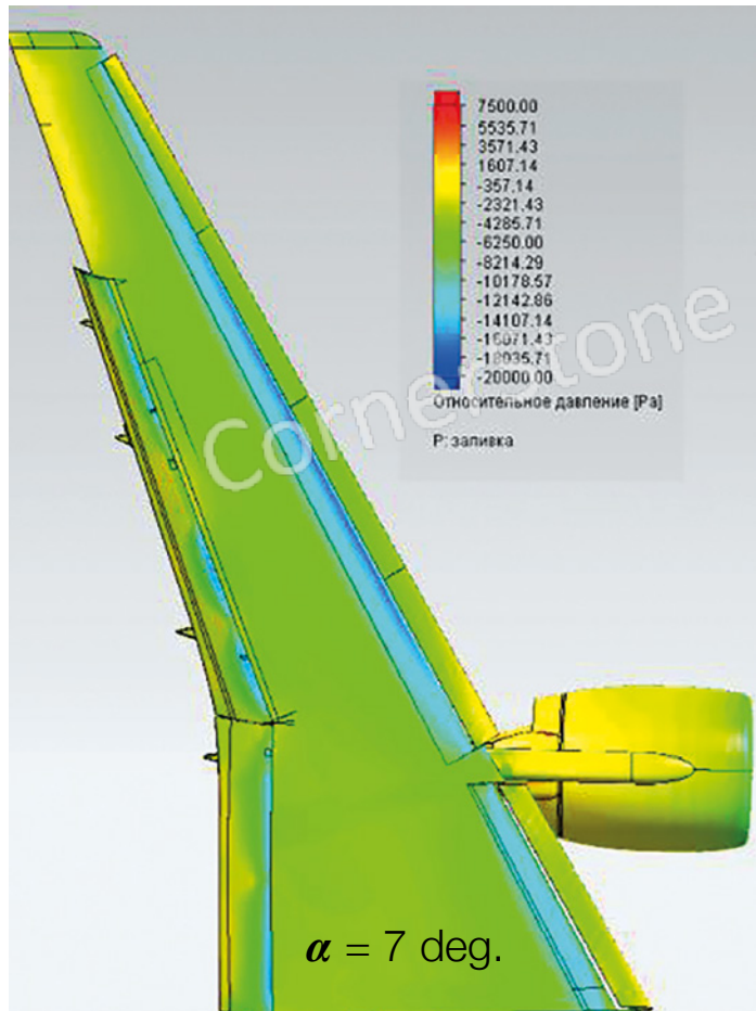
Figure 4. Computation Results: \Delta P on Wing Surface
