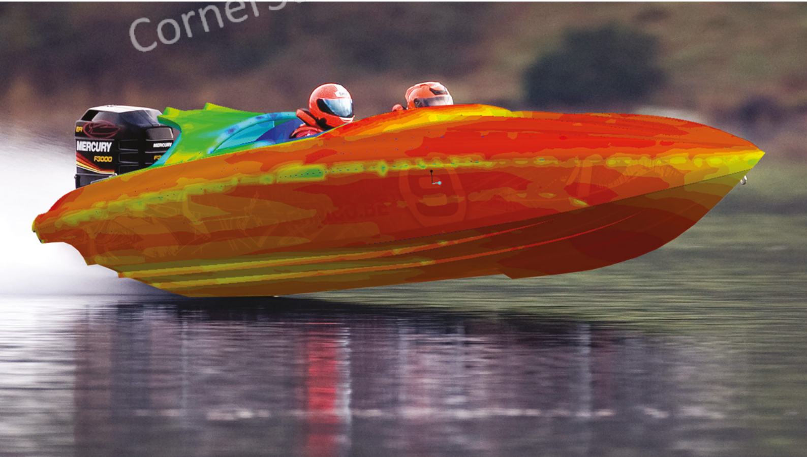
Figure 4. Record Breaking F2 Bernico Boat on Coniston Water in November 2009 with superimposed hull pressure contours from FIoEFD simulation prediction
