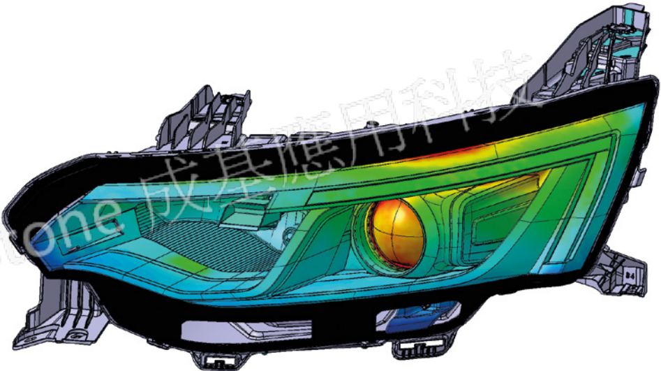
Figure 6: FloEFD Thermal Predictions for a Renault Halogen Headlamp Assembly
