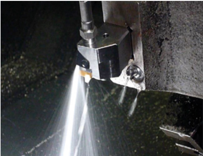
Figure 9. Final JT Holder Nozzle Spray Configuration
