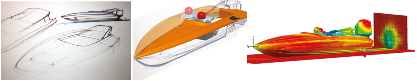
Figure 1. Voxdale F2 Speed Boat Design Process - Brainstorm & Conceptual Design (left) Architecture & SDX (center) and Engineering & Optimization (right) - Pro/E, ISDX, AAX, FloEFD
