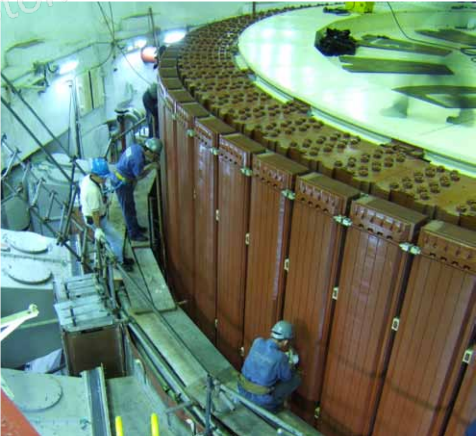
Figure 1. Rotor of a Hydro Generator. Photo courtesy of Hydropower Consult
