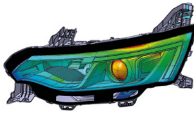
Figure 1. Renault Laguna Headlight assembly thermal analysis (left) in FloEFD and airflow pathline details (right)
